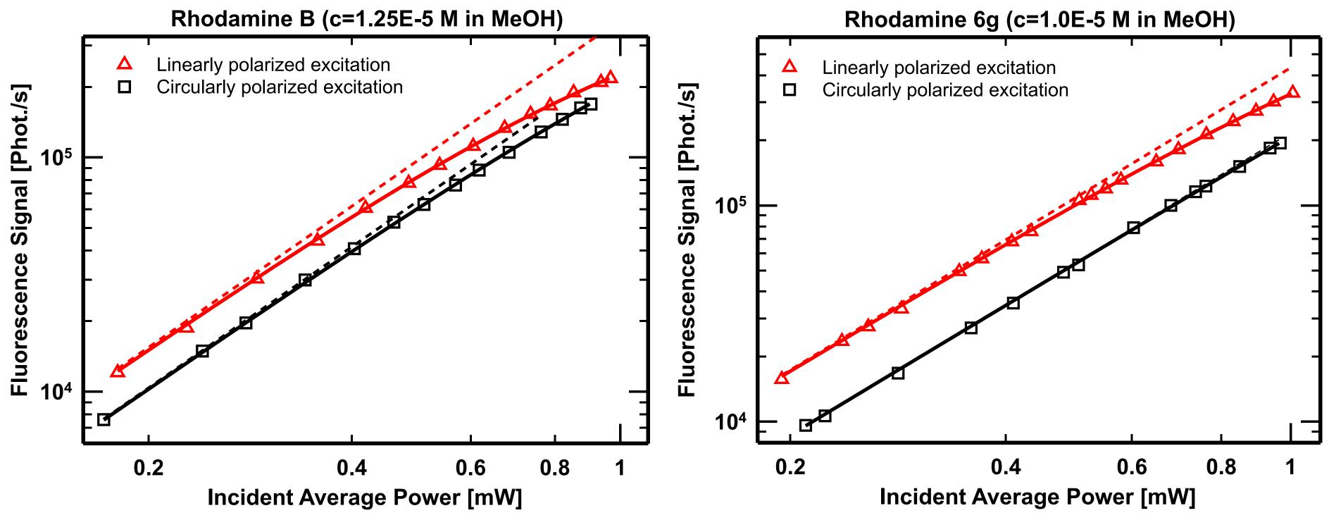
Log-log plot of the dead-time corrected fluorescence signal at different laser average power
